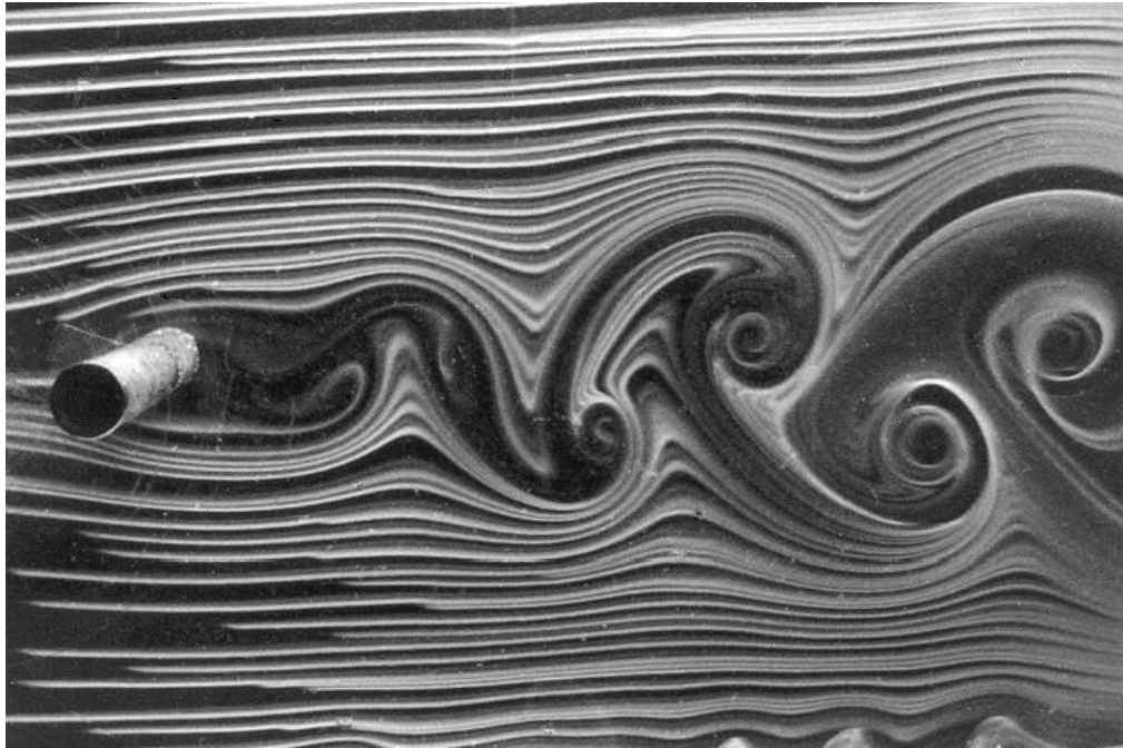
Karman vortex sheet: repeating swirling vortices caused by unsteady separation of flow of a fluid around blunt bodies.
